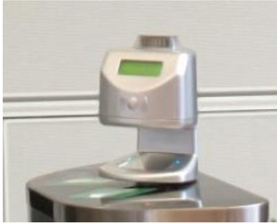
*OpenPark TT is a ticketing terminal specially designed for leisure applications such as stadiums, fun parks, aqua parks, fitness centers, zoo parks etc. This terminal is developed to read a variety formats of barcodes, QR codes, RFID cards and wristbands. OpenPark TT can ensure a large internal memory for off-line ticket verification in case of communication failure and anti-passback feature.*
